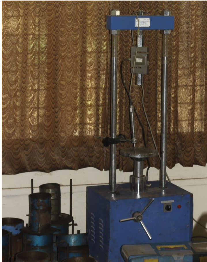
California Bearing Ratio (CBR) Test Apparatus
