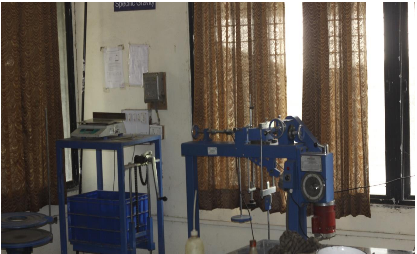
Buoyancy Balance Apparatus for determining Specific Gravity of Soils
