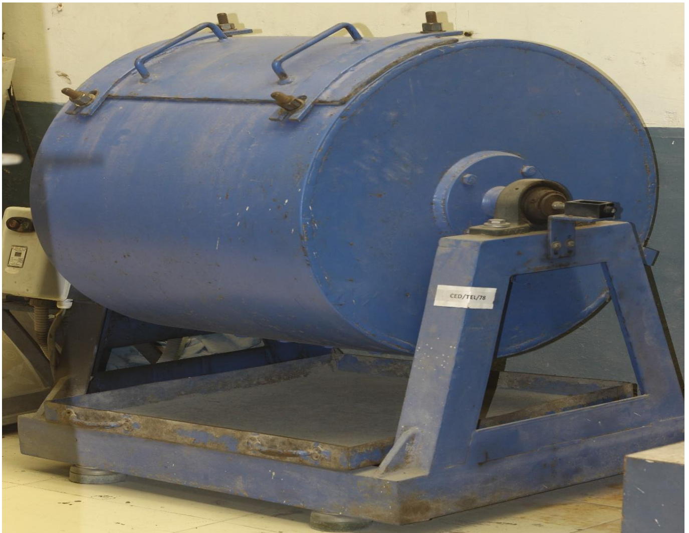
Los Angeles Abrasion Testing Machine for testing Aggregates
