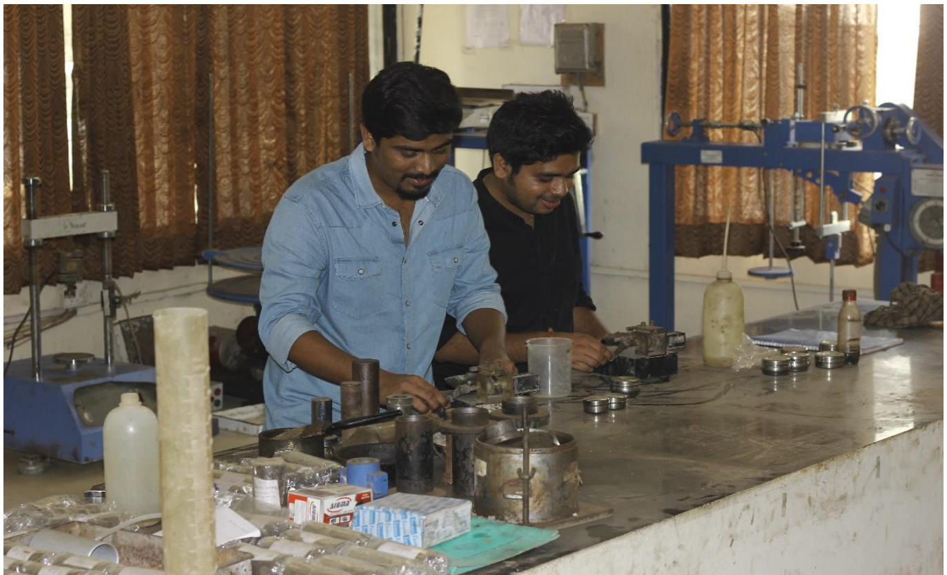
M. Tech I Year Students Performing Experiment of Liquid and Plastic Limit of Soil
